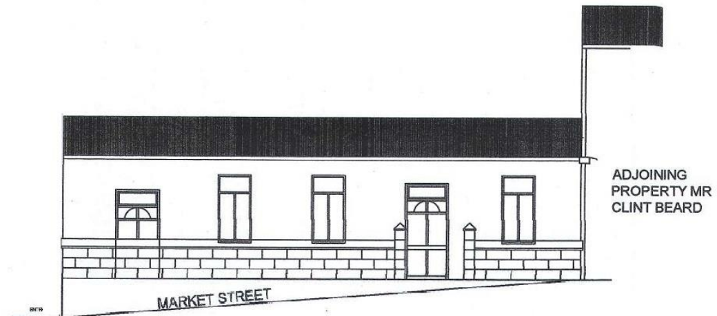
FRONT ELEVATION SHOWING PROPOSED NEW UPVC COATED ALUMINIUM WINDOWS
