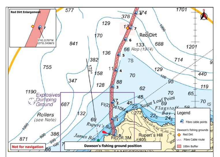
Below is the position track of the cable, running from the shore to approximately 7km out to sea, if you wish to put it in a chart potter or handheld GPS:
