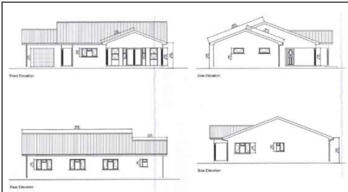
The roof will be of a gable design covered in IBR sheeting, and the external walls constructed out of concrete blockwork. In terms of the sewerage, this will be connected into a septic tank soakaway system.
