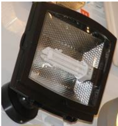
Poor – Low wattage light source but projects light upwards when mounted as shown and needs to be near horizontal to limit sky glow. (Bracket does not allow horizontal fixing) 18 watt PL-C = 1,200 lm
