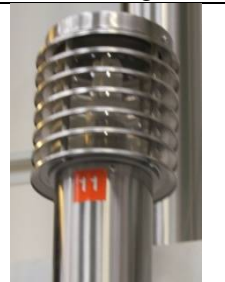
Fair – External louvers limit some upward light and reduces glare. Lamp must be less than 500 lm
