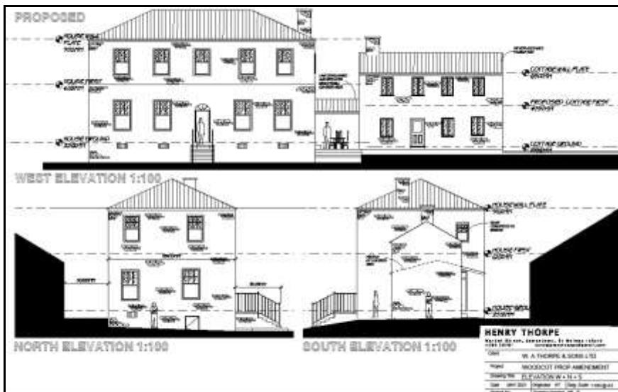
On the MAIN BUILDING, it is also proposed to remove the proud cement pointing and repoint with lime mortar. The existing cement mortar was applied in recent years and stands out from and overpowers the stone wall. The proposed lime mortar will be flush with the stone and struck with a stipple brush therefore returning the building to its original state.
