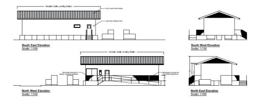
3.5 The need was change in design was prompted by the development for the Container Freight Development to enable the Port Security Officer to have clear line of vision of the Wharf Area from the first floor observation. The Cable Landing station roof level was obscuring the line of vision. The roof design now proposed overcome this issue and it is considered that the proposal does not in any way compromises the design aesthetic.
