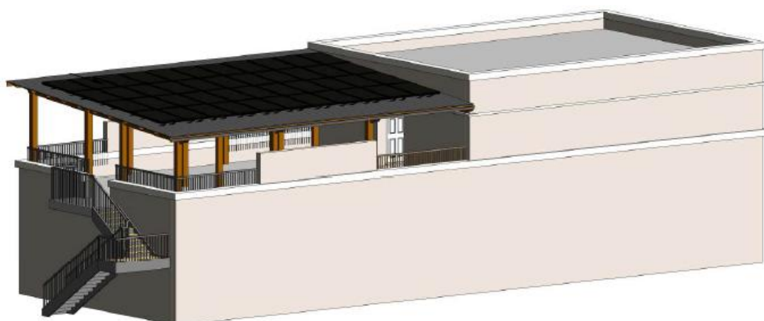
Diagram 9: Proposed Pergola With PV Panels – 3D Perspective
