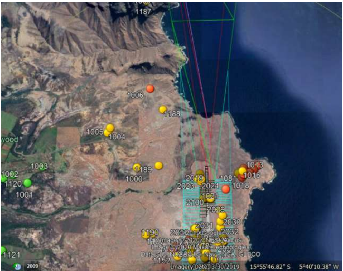
Figure 5 – Wedge shaped area originating at the departure and arrival end of the runway and extending for 3 nautical miles from the runway over which the aircraft would normally track
