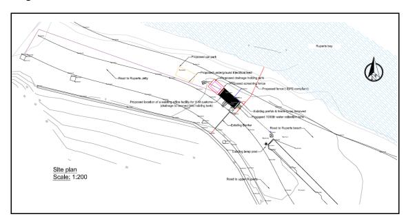
In order to accommodate the office, the existing prefabricated hut and fence will be removed. The office will then be sited on the north eastern corner of the barrier. The floor layout consists of an office and kitchenette area. An intervening lobby will separate the office from the toilet.
