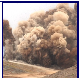
9. Blast takes place, moving thousands of tons of rock
