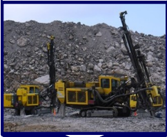
1. Holes drilled for blasting grid
