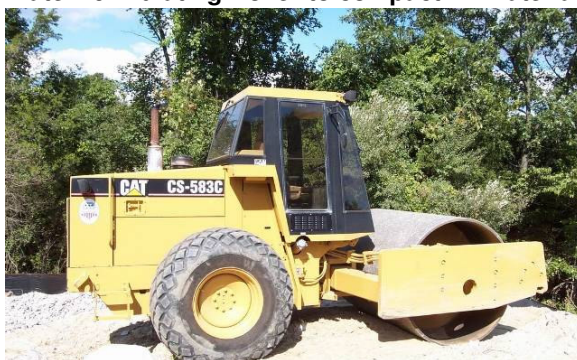
Plate 2.9 Vibrating Roller to compact fill material
