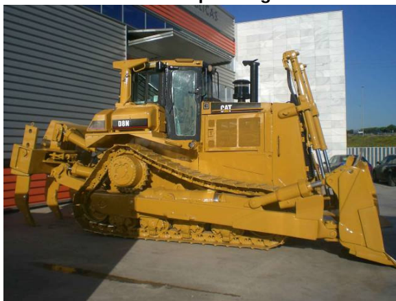
Plate 2.8 Bulldozer for spreading fill material
