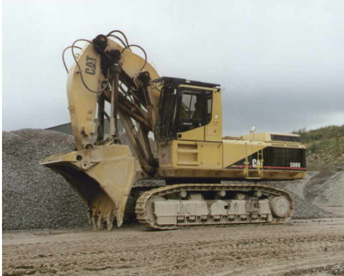
Plate 2.6 – Dump Truck Loading Shovel for Excavating Fill Material
