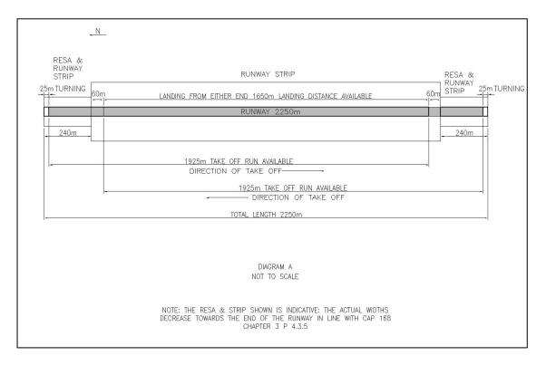
Note: In these diagrams, the 25m turning distances are included in the term 'runway' as paved areas, although separately shown as non-shaded elements.
