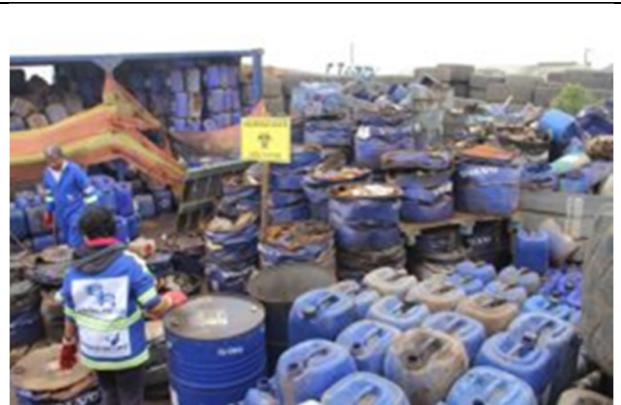
Plate 31: Drums containing oil filters after having been compacted. Note that the jerry cans cannot be effectively compacted and still take up excess storage space before being cleaned.
