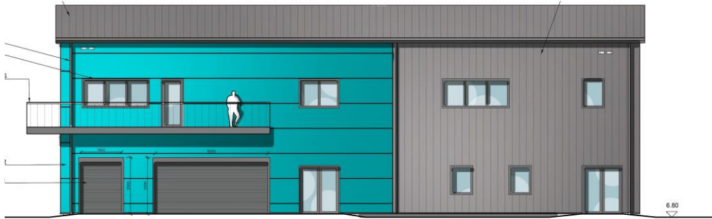
Diagram 8: Main Elevation of the Port Control Building
