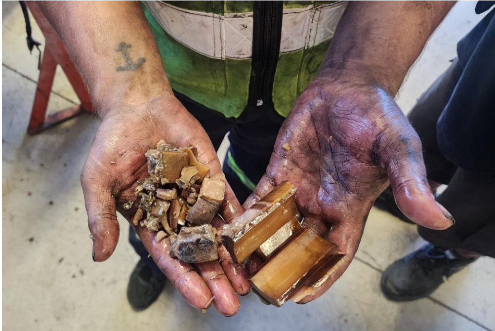
Figure 32: Damage to R3 eccentric (3)
