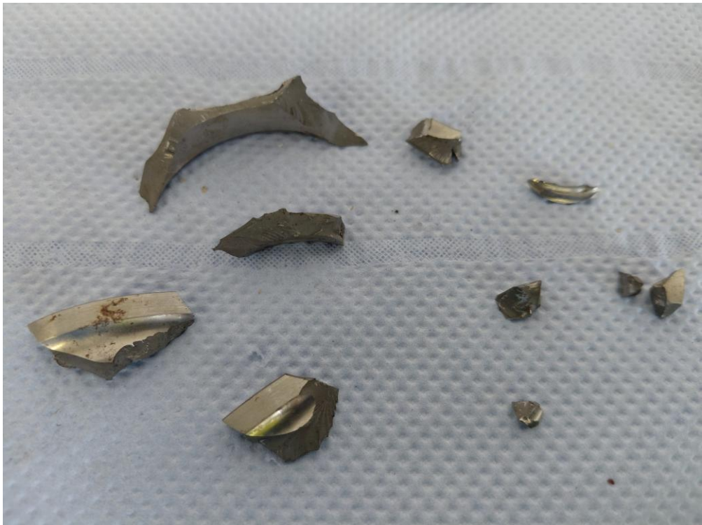
Figure 80: Inspection of R2 gearbox bearing (3)
