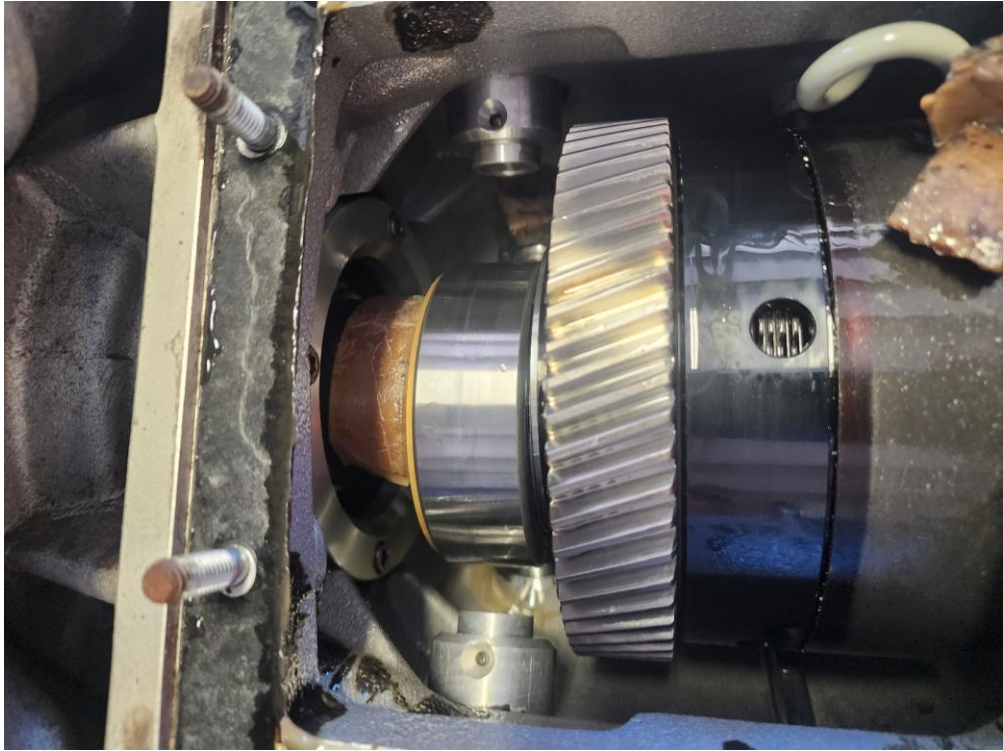
Figure 30: Damage to R3 eccentric (1)
