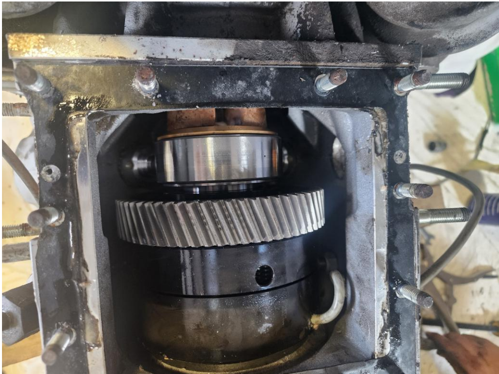
Figure 26: Damage to R1 eccentric (1)
