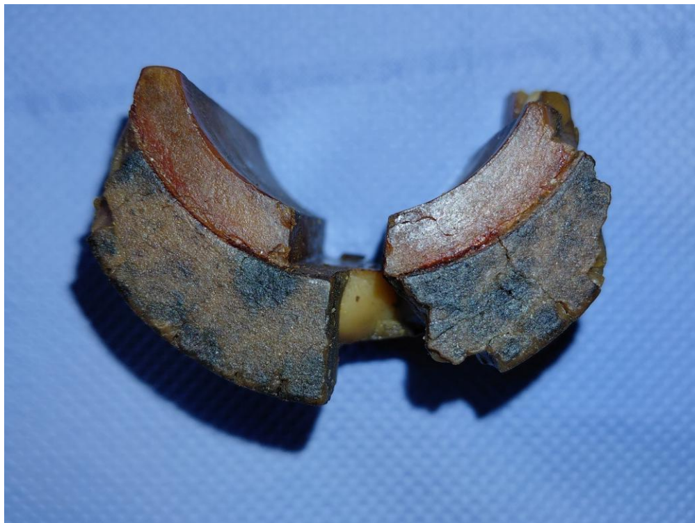
Figure 44: Inspection of R1 eccentric (9)
