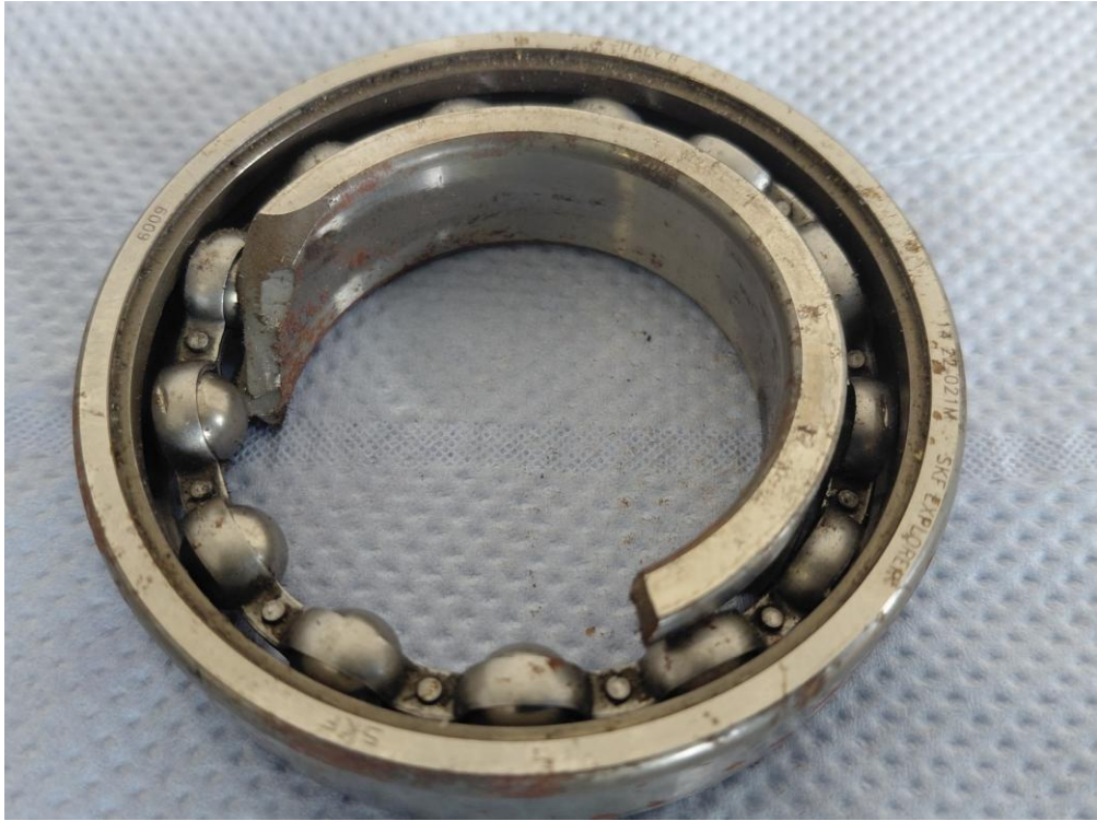
Figure 79: Inspection of R2 gearbox bearing (2)
