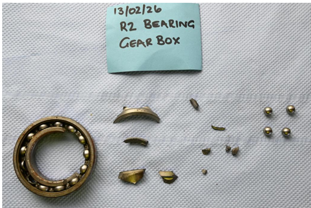
Figure 78: Inspection of R2 gearbox bearing (1)
