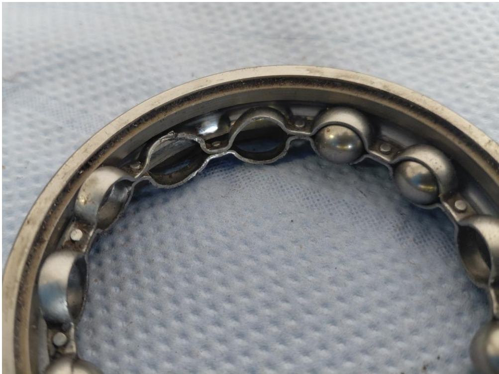
Figure 86: Inspection of R2 gearbox bearing (9)
