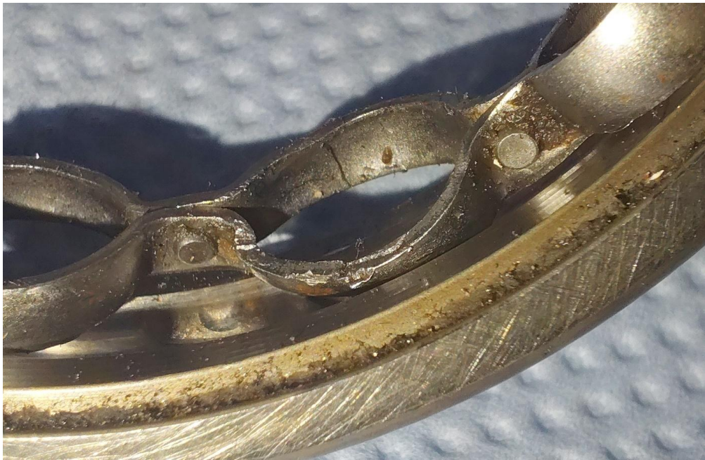
Figure 88: Inspection of R2 gearbox bearing (11)
