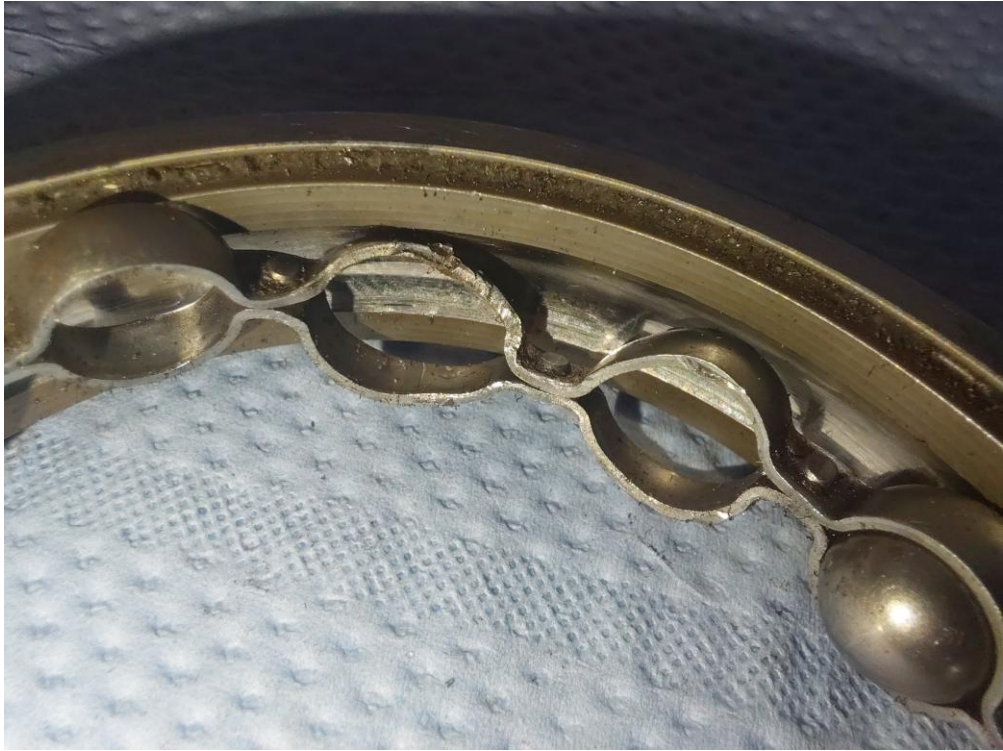
Figure 87: Inspection of R2 gearbox bearing (10)
