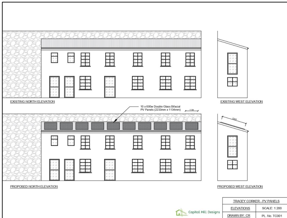
Diagram 2: Existing & Proposed North & West Elevations
