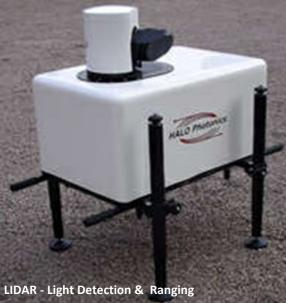
LIDAR (Light Detection and Ranging), has now been installed for St Helena Airport. It is a remote sensing method that uses light in the form of a pulsed laser to measure distances and has many applications, from 3D mapping of terrain from aircraft, to modelling archaeological sites, to helping autonomous cars avoid obstacles - it is even the basis of police speed guns.
