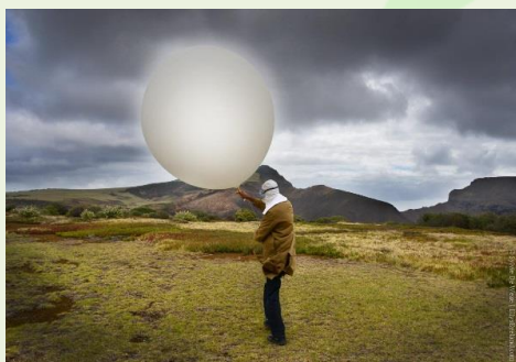
Preparing & launching of the 'Totex TX800' Weather Balloon with attached Vaisala Radiosonde RS92
